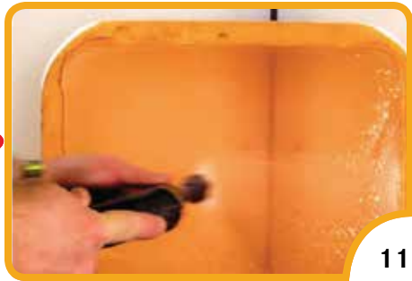
High-pressure rinse from bottom to top
