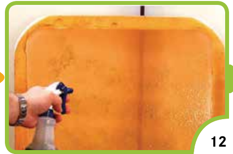
Apply SAATI Chemicals Direct Prep to one side of screen, brush both sides
