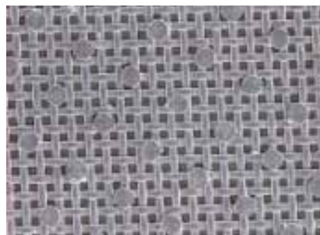
SAATI HiBond Plus halftone area with no stencil loss
