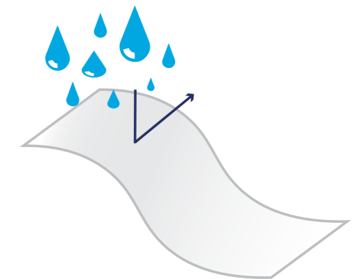
The hydrophobic treatment protects the filter media against liquids such as water
