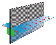
The mesh can be defined as **Neutral** if the contact angle is right at  $90^{\circ}$
