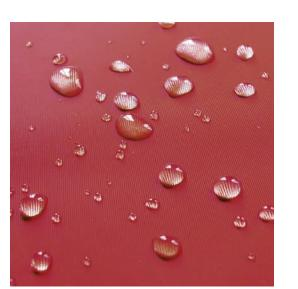
The mesh can be defined as Hydrophobic if the contact angle is higher than 90  $^\circ$
