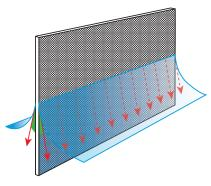
The mesh can be defined as Hydrophilic if the contact angle is lower than  $90\,^\circ$
