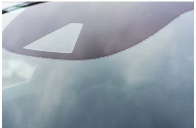
Screen printed rain sensors on front window.
