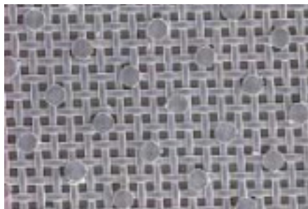
SAATI HiBond Plus halftone area with no stencil loss
