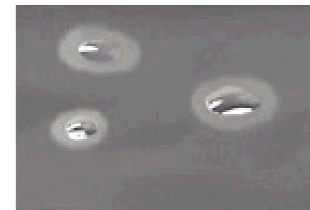
Water droplets on fabrics with plasma treatment
