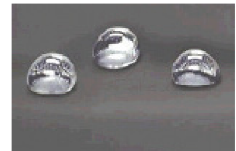
Water droplets on convential fabrics
