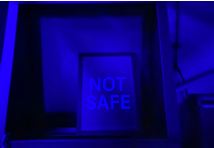
Top: An example of the light in screen rooms with standard flourescent tube or LED lighting Bottom: Light visible through the Safe Light Glasses shows the elevated presence of light wavelengths that affect photosensitive emulsions and films
